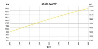
All power levels are stated gross kilowatts per SAE J1940 as rated by Briggs & Stratton.
