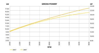
All power levels are stated gross kilowatts per SAE J1940 as rated by Briggs & Stratton.
